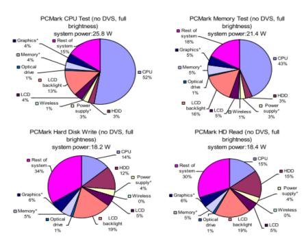
Figure 1: Power Consumption under different workloads
